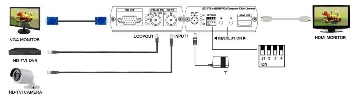
\* 3 outputs: HDMI, VGA, HD-TVI loop output as a distributor.
