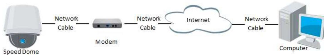
Figure 2-6 Accessing the Speed Dome with Dynamic IP
